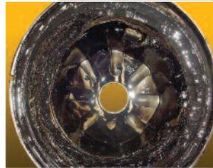
*Centrifuge bowl containing 2.4 pounds of contaminants removed from the oil during the test period.*
