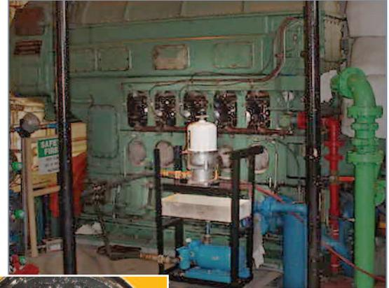
*Engine with Spinner II centrifuge on test stand.*
