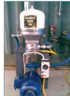
Spinner II Model 3400 centrifuge test unit
